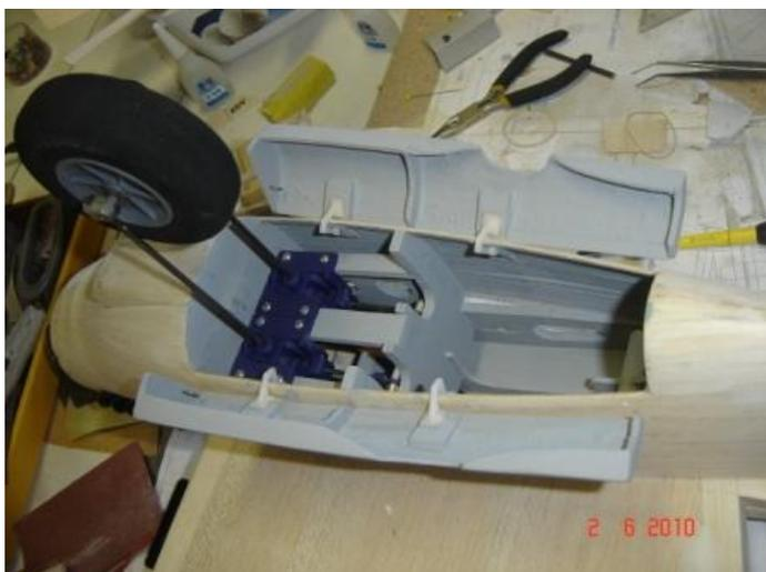
All's well I thought, now for the retract doors. Normal hinges won't work here because the doors are curved in 3 dimensions, so I bought some offset hinges which allows the doors to move whilst increasing the gap.
