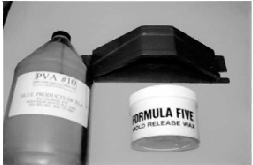
Step 4. Four coats of mold release wax are applied and polished, one hour between coats, then four coats of PVA are brushed or sprayed on to ensure clean release.
