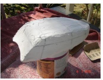
but make one like the Spit, looks o/k when it's in the air. I tried a couple of ideas but ended up carving one out of a couple of pieces of polystyrene blocks glued together. I don't have any dimensional drawings so
