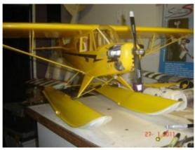
I covered the mostly desperate maiden flight on the VRCMC 'Have Your Say" page a couple of weeks ago and since then I've made a couple of adjustments to stop the severe tendency to turn left. Re aligning the RH float which Colin pointed out to me. The Cub last flew on my Futaba 6ch radio and after checking the settings the aileron right trim was set to 80%, hadn't put that into my new radio. Now all we need is some good weather and we can try a second flight.
