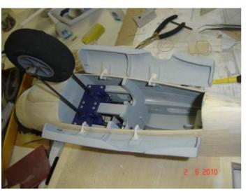
All's well I thought, now for the retract doors. Normal hinges won't work here because the doors are curved in 3 dimensions, so I bought some offset hinges which allows the doors to move whilst increasing the gap.
